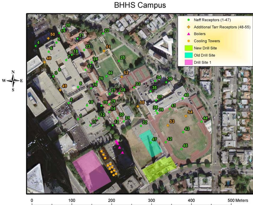
Figure 2-2: Map of Beverly Hills High School (BHHS) showing location of facilities along with 47 receptors used by Dr. Neff to calculate concentrations in his wind tunnel simulations.
