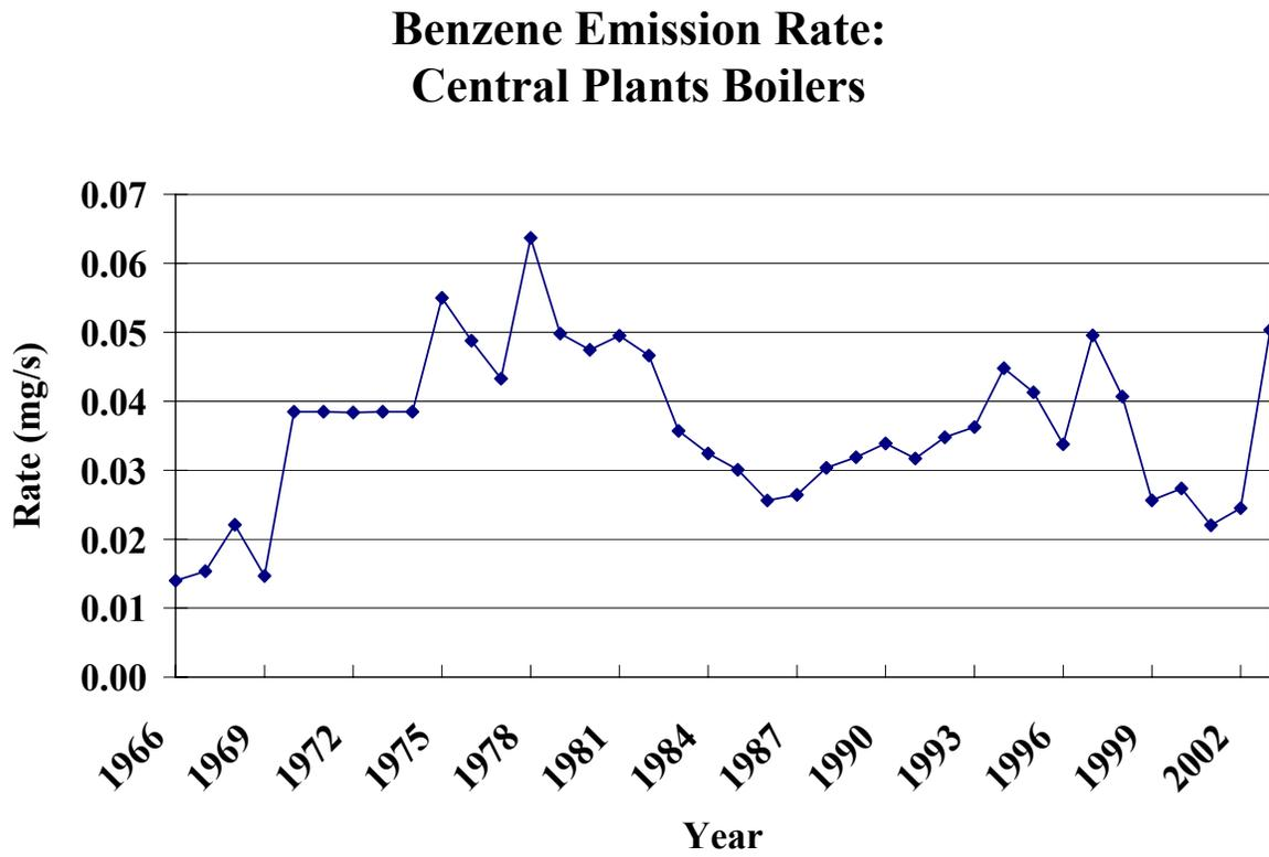
Figure 5-5: Benzene emission rates versus year from Boilers, as supplied by Sierra Research.
