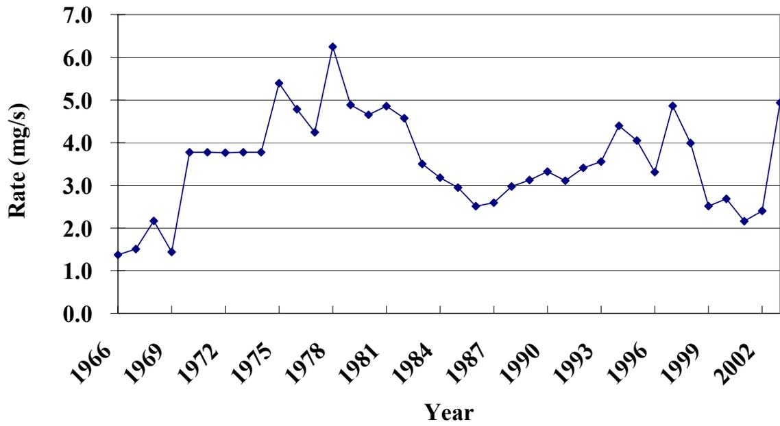
Figure 5-6: Formaldehyde emission rates versus year from Boilers, as supplied by Sierra Research.
