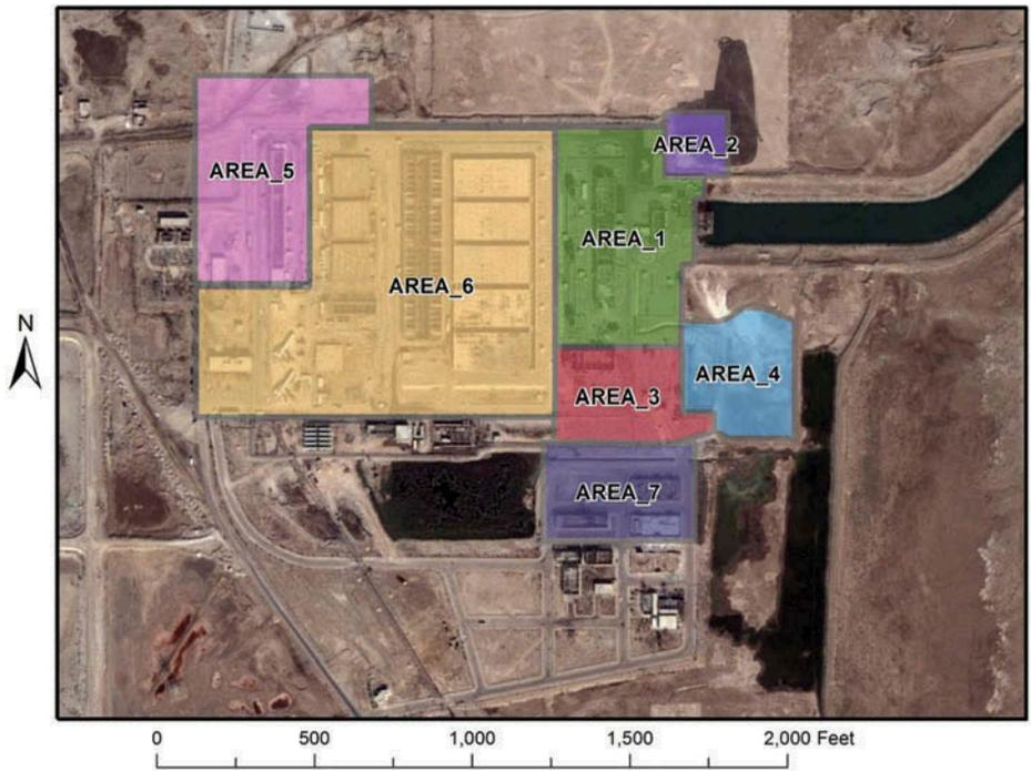
Figure 10. Seven areas across the Qarmat-Ali WTP used to characterize average Cr(VI) soil concentrations and associated Cr(VI) air emissions in modeling.
