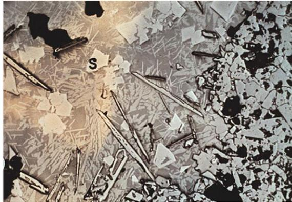
**Figure 10: Microstructure at the immediate Slag/Brick Interface (130X)**
