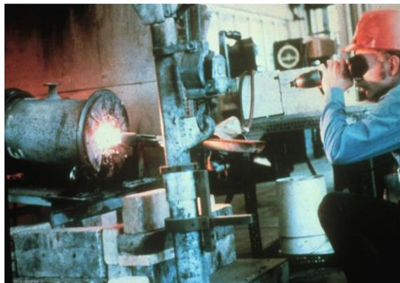
**Figure 32: Rotary Slag Test for Refractories**
