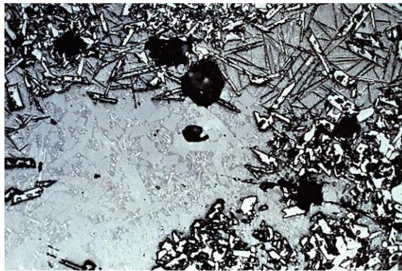
**Figure 11: Position Where Mullite Crystals Appear Behind The hot Face**
