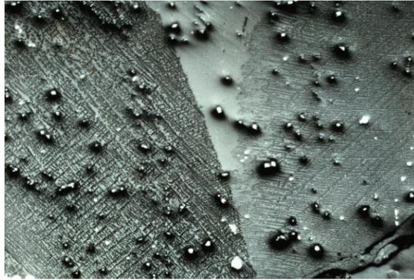
**Figure 25: AOD reduction Slag (130X)**
