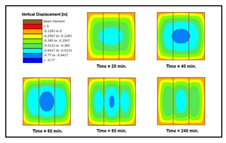
Using PBSFD, engineers can predict the behavior of a frame in fire, such as vertical displacement of floor beams over time.
