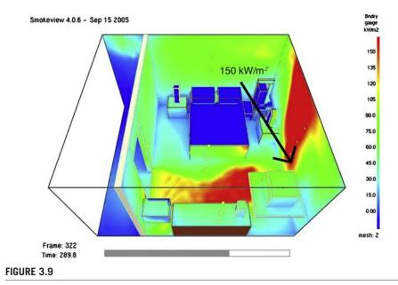
Output of a fire dynamics simulator computer program used to model the Las Vegas test fire. Because of the influx of oxygen from the doorway, a large, but not terribly meaningful fire pattern developed on the opposite wall.
