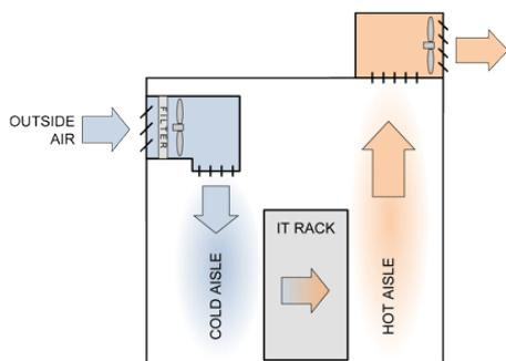
**Air-Side Economization** at its simplest level involves using outside air to cool the data center. There are many ways to do this, with varying levels of complexity. Simply opening doors and windows would be a form of air-side economization (although not a particularly effective or secure one). The image at left shows a simple example of air-side economization. More complex approaches can utilize evaporative cooling, indirect air handling with air-to-air heat exchange, and many more.
