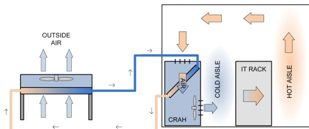
**Water-Side Economization** is applied to systems which use water to transfer heat away from the data center. In its simplest form, cool water passes through the coil in the CRAH unit and picks up heat from the warm data center return air. This warmed water is sent to an outdoor cooler (dry cooler or cooling tower) where the heat is removed and the cooled water is sent back to the CRAH unit.
