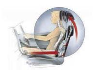
An active head restraint moves forward and upward in a rear-end collision to decrease the space between the restraint and the occupant's head. By doing so, the dynamic restraint reduces the degree to which the head accelerates before making contact. By reducing the acceleration, the potential of occupant injury is decreased. Active head restraints are devices typically applied to a vehicle's front seats, but can also be found in rear seats as well.
