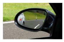
Side View Assist/Blind-Spot Warning technology operates similar to the Reverse Warning Sensors but incorporates side-mounted sensors. Driver notification is typically accomplished via activation of a warning lamp located in the side-view mirror on the side of the potential hazard.
