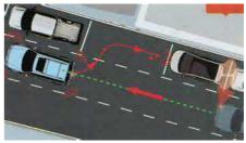
maneuvers. Electric Steering Assistance operates only when required, thus reducing fuel consumption. Electric Steering Assistance can also be programmed to self-steer. Together, with side and rear-mounted sensors, Electric Steering Assistance, and programming algorithms, Parking Assist temporarily takes control of vehicle steering, and other vehicle systems, in order to self-park the vehicle.
