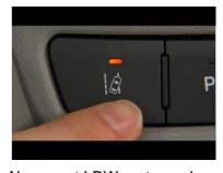
markings, it can potentially lead to false alerts. Also, most LDW systems do not operate at speeds less than approximately 30 miles per hour.
