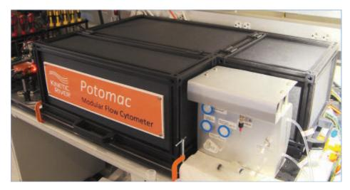
**FIGURE 4.** The Kinetic River Potomac modular flow cytometer has an architecture designed for open access. This unit, installed at the National Cancer Institute, was customized to work with external lasers.
