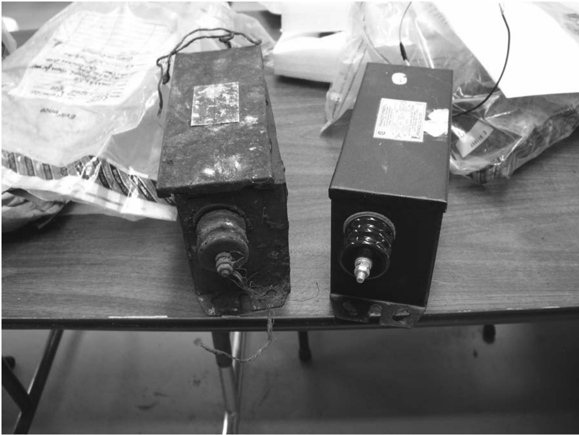
Figure 5 - Recovered and new neon transformers
