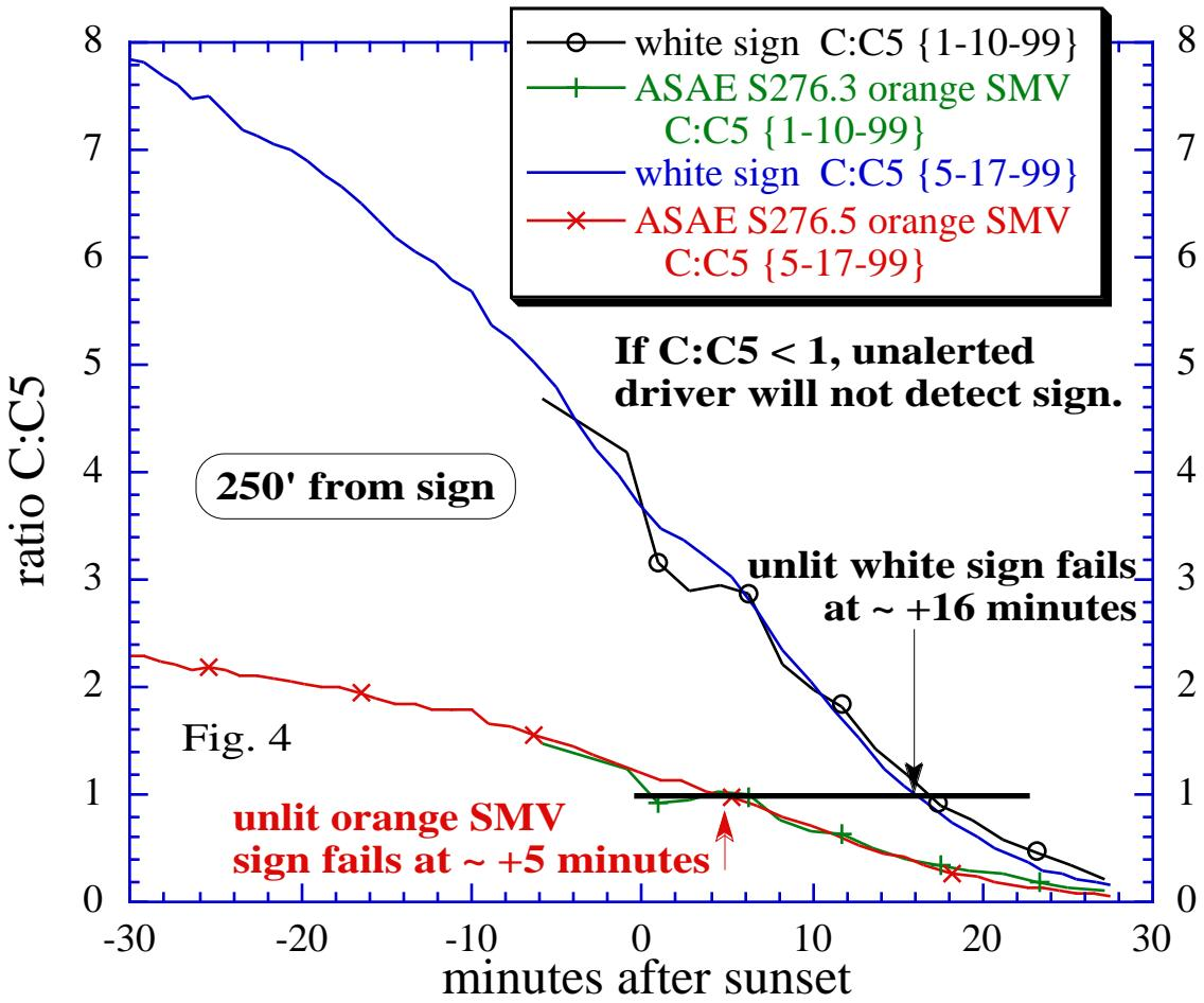
Figure 4: The data of Fig. 3 redrawn using the ratio C:C5 vs. time after sunset (alternatively, time before sunrise), and now including trends for both a wintertime and summertime sunset. A white sign ( $R = 90\%$ ) that is lit only by skylight could attract the attention of an unalerted driver at 250' until about 16 minutes after sunset, while an orange SMV sign would first fail to do so at 5 minutes after sunset.
