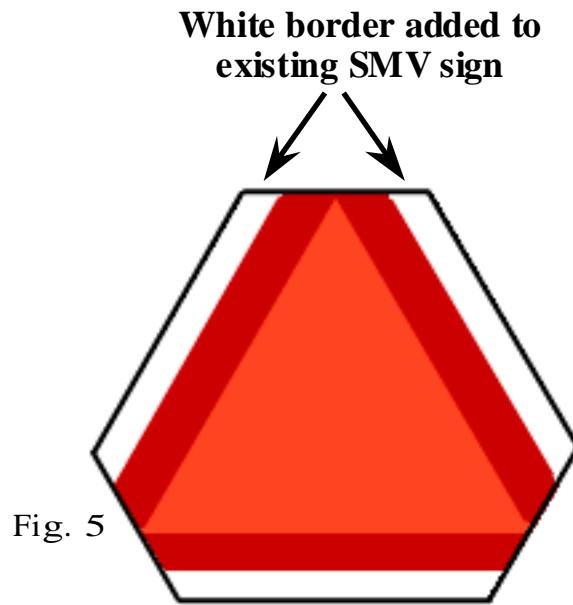
Figure 5: One possible alternative to the current SMV sign simply adds a white border to it, thereby preserving the sign's shape while increasing its size (and thus its visibility). In principle, this more reflective SMV sign would be detected more easily by those drivers whose headlights are off during civil twilight.
