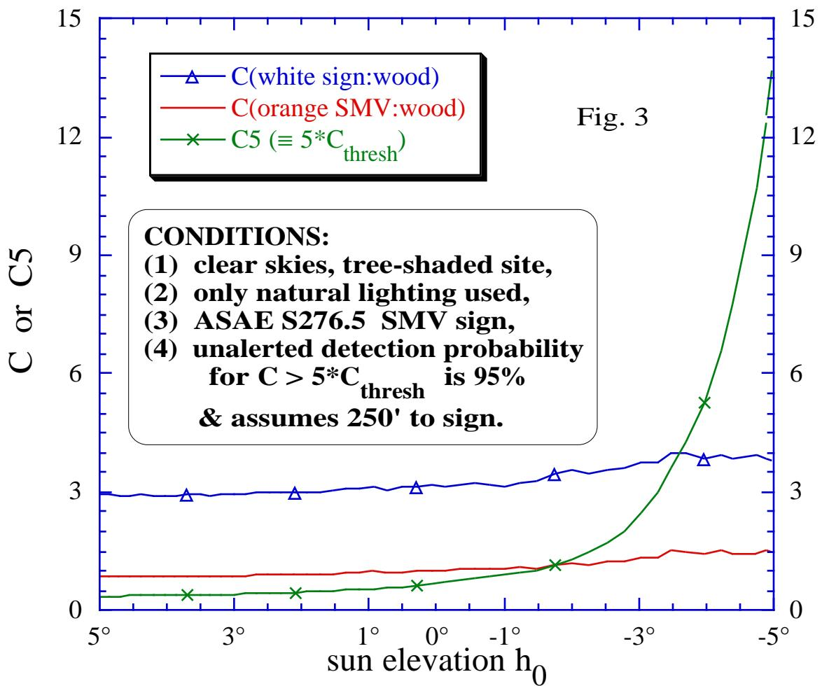
Figure 3: Luminance contrast  $C$  for a white sign and for SMV orange against a wood background, plotted as functions of unrefracted sun elevation  $h_0$ . A fivefold multiple of the variable contrast threshold  $C_{\text{thresh}} (\equiv C5)$  is shown as the curve with xs. Although  $C$  increases slightly after sunset,  $C5$  increases much more, making both the white and orange signs progressively more difficult to detect.
