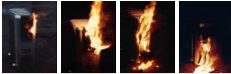
FIGURE 2 BELOW: IGNITION TEST, PLASTIC TRIM OF PORTABLE ELECTRIC HEATER
