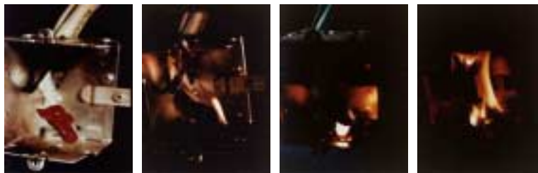
FIGURE 4 BELOW: BURN TEST, CONNECTOR INSULATING SHELL
