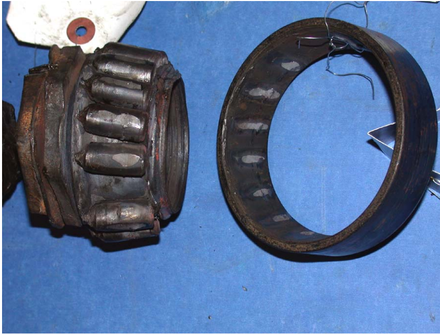
Figure 1: Outer bearing from spindle #10. Rollers are welded to the inner race.
