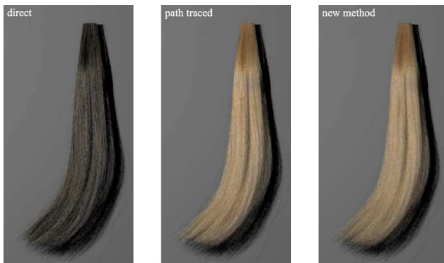
Figure 31: Rendering results of a ponytail lit from the front. (left) Single scattering result. (center) Path tracing results after 60 hours (right) Moon and Marschner’s photon map based approach in 2.5 hours. From [Moon and Marschner 2006].
