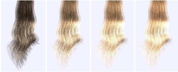
Figure 30: Rendering an assembly of blond hairs with Zinke’s shading model and increasing the depth of scattering from 1 (left) to 4 (right). From [Zinke et al. 2004].
