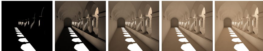
Figure 5. ICPT used for rendering our diffuse Sponza scene with 0, 1, 2, 3 and 4 bounces of indirect illumination with 4K samples per pixels. Indirect illumination is essential for rendering this scene.
